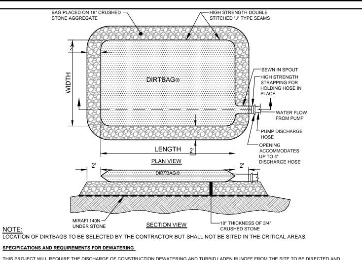
THIS PROJECT WILL REQUIRE THE DISCHARGE OF CONSTRUCTION DEWATERING AND TURBID LADEN RUNOFF FROM THE SITE TO BE DIRECTED AND DISCHARGED THROUGH A DIRTBAG. THIS DESCRIPTION ALSO CONTAINS APPENDED MATERIALS DESCRIBING THE DIRTBAGS REFERRED TO IN THIS NARRATIVE
