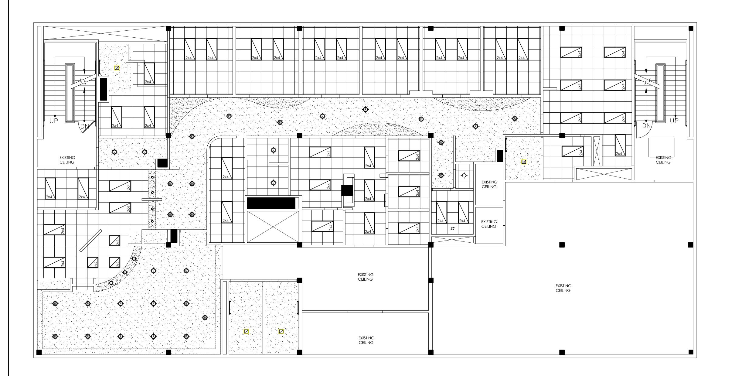
CEILING LEGEND \*ALL EXIT AND EMERGENCY LIGHTS ARE THE RESPONSIBILITY OF THE LIGHTING CONTRACTOR AND TO BE INSTALLED PER LOCAL CODE. \*GENERAL SWITCH LOCATIONS AND WIRING TO BE DETERMINED BY LIGHTING CONTRACTOR PER LOCAL CODE AND BE APPROVED BY DOCTOR. SUSPENDED CEILING GRID GYP. BRD. CEILING OR SOFFIT. CONFIRM HEIGHTS WITH HENRY SCHEIN REP. CEILING MOUNTED LIGHT FIXTURE  $\sigma$ EXHAUST FAN VENTED TO OUTSIDE **®** RECESSED LIGHT FIXTURE **P** PENDANT LIGHT FIXTURE WALL SCONCE MIRROR LIGHT
