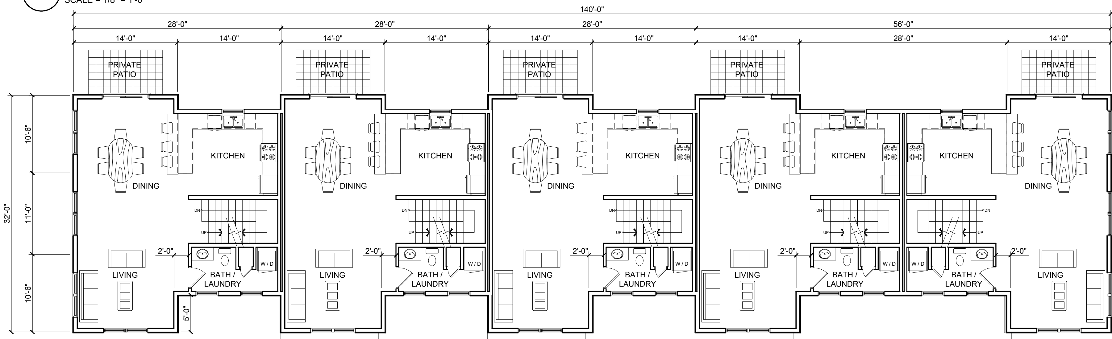
3 SECOND FLOOR PLAN SCALE = 1/8" = 1'-0"
