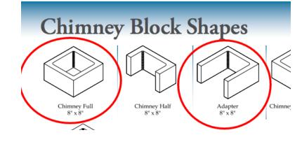
Double chimney will be built using Genest Concrete Chimney Blocks. Each course will use one 8x8 chimney full and one 8x8 adapter, alternating on the way up. This creates two 8x8 chambers separated by 4", as code requires.
