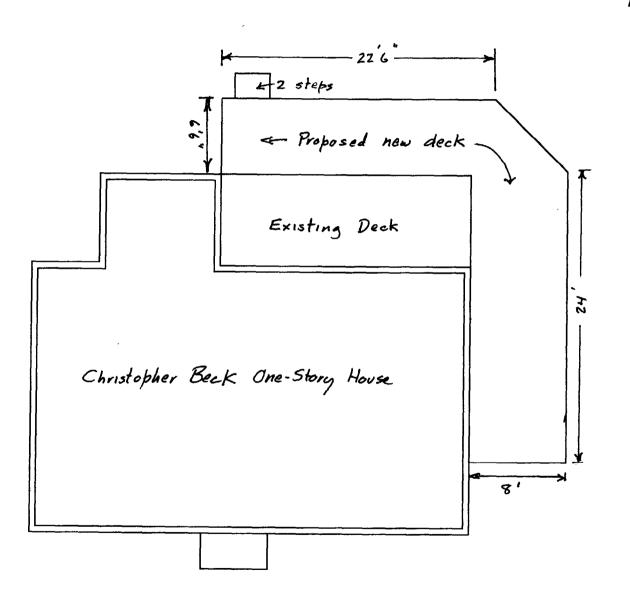
Note: Existing deck has been dismantled due to rot and potential failure. Leaks at old ledger board repaired. Proposed new deck will include rebuilding of old ("existing") deck.
