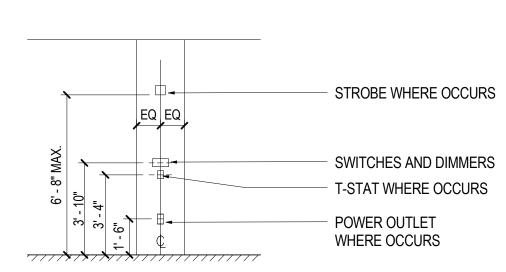
LOCATIONS at COLUMNS, BETWEEN DOORS, ETC. **SWITCHES, STROBES and THERMOSTATS**
