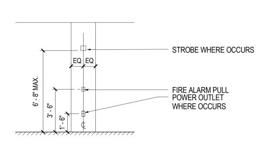
11 LOCATIONS at COLUMNS, BETWEEN DOORS, ETC. **OUTLETS, STROBES and FIRE ALARM PULLS**
