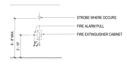
LOCATIONS at FIRE EXTINGUISHER CABINET STROBES and FIRE ALARM PULLS
