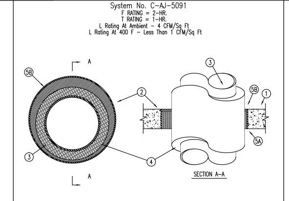
1. Floor or Wall Assembly — Min 4-1/2 in. thick reinforced lightweight or normal weight (100-150 pcf) concrete. Wall may also be constructed of any UL Classified Concrete Blocks\*. Max diam of opening is 20 in. See Concrete Blocks (CAZT) category in the Fire Resistance Director for names of manufacturers.
