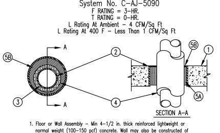
any UL Classified Concrete Blocks\*. Max diam of opening is 8 in. See Concrete Blocks (CAZT) category in the Fire Resistance Directory for names of manufacturers.
