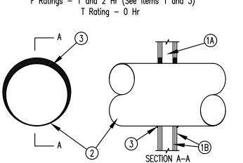
1. Wall Assembly The 1 or 2 hr fire rated wallboard/stud wall assembly shall be
