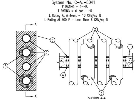
1. Floor or Wall Assembly - Min 4-1/2 in. thick reinforced lightweight or normal weight (100-150 pcf) concrete floor or min 5 in. thick reinforced lightweight or normal weight (100-150 pcf) concrete wall. Wall may also be constructed of any UL Classified Concrete Blocks\*. Max area of opening is 192 sq in. with max dimension of 24 in.
