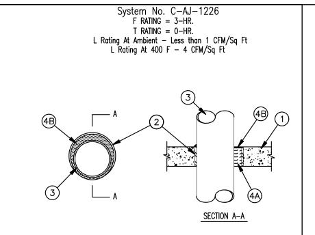
1. Floor or Wall Assembly -- Min 4-1/2 in. thick reinforced lightweight or normal weight (100-150 pcf) concrete. Wall may also be constructed of any UL Classified Concrete Blocks\*. Max diam of
