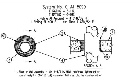
any UL Classified Concrete Blocks\*. Max diam of opening is 8 in. See Concrete Blocks (CAZT) category in the Fire Resistance Directory for names of manufacturers. 2. Metallic Sleeve (Optional) — Nom 8 in. diam (or smaller) Schedule 10 (or heavier) steel pipe.
