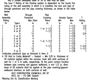
System No. W-L-7040 F Ratings - 1 and 2 Hr (See Items 1 and 3) T Rating — 0 Hr 1. Wall Assembly - The fire-rated gypsum wallboard/stud wall assembly shall be constructed of the materials and in the manner specified in the individual U300 or U400 Series Wall and Partition Designs in the Fire Resistance Directory and shall include the following construction features:
