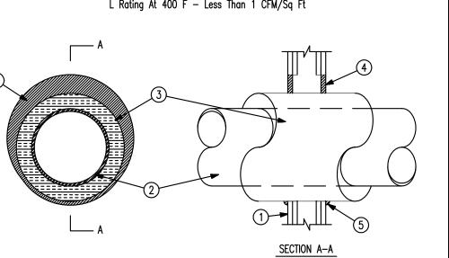
1. Wall Assembly - The 1 or 2 hr fire-rated gypsum wallboard/stud wall assembly shall be constructed of the materials and in the manner in the UL Fire Resistance Directory and shall include the following A. Studs - Wall framing may consist of either wood studs or steel channel studs. Wood studs to consist of nom 2 by 4 in. lumber space 16 in. OC. Steel studs to be min 2-1/2 in. wide and spaced max 24 in.
