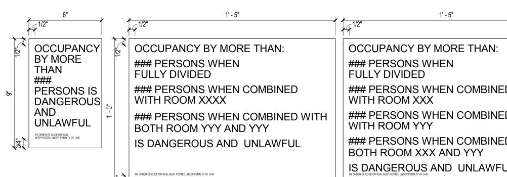
CONTROLLING DIMENSION IN ANY OF THE CODES FOR THE LETTERING SIZE OR THE SIZE OF THE SYMBOL OF ACCESSIBILITY. 5/8" WOULD BE THE MIN HEIGHT FOR THE TEXT
