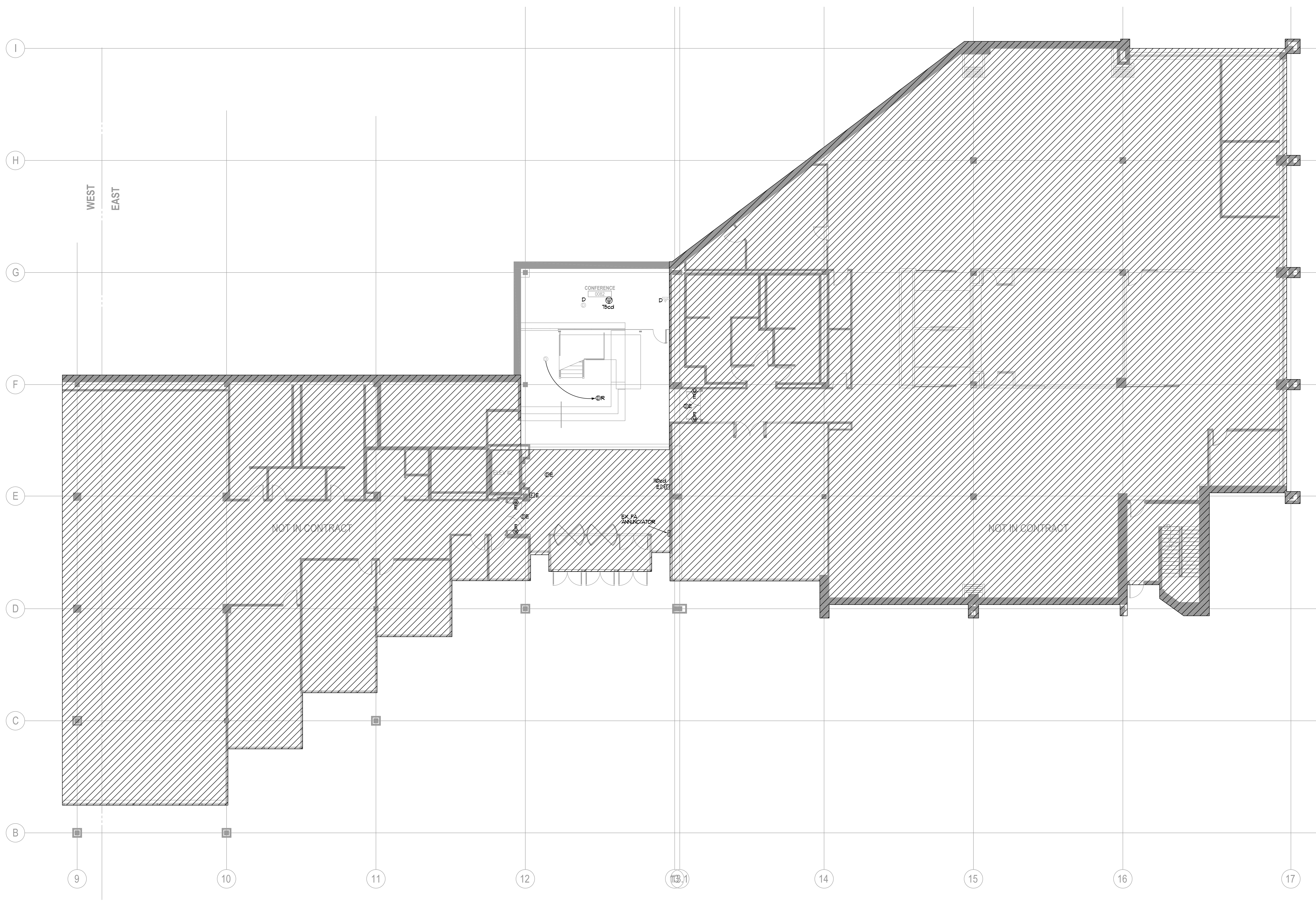
E1.300E GROUND FLOOR PLAN (EAST) - FIRE ALARM 1/8" = 1'-0"
