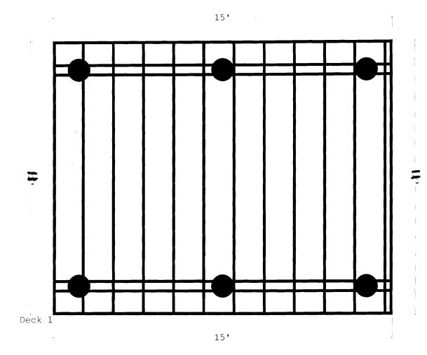
Joist Spacing = 16 in. o.c. Baluster Spacing = 3 3/4" Toe Spacing = 3 3/4" Railing Height = 36" The Home Depot # 2406 300 CLARKS POND PKWY, S PORTLAND, ME 04106 (207) 879-2500 Wed Aug 15 12:44:52 2007 THUY NGUYEN DECK 148187
