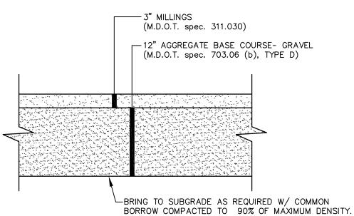
1. COMPACT GRAVEL SUBBASE, BASE COURSE TO 92% OF MAXIMUM DENSITY USING HEAVY ROLLER COMPACTION.
