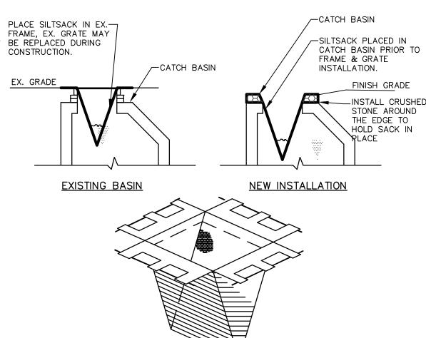
SILT SACK PROTECTION PRIOR TO FINAL GRADING AND PAVING OPERATIONS BEGIN A CATCH BASIN INSERT (SUCH AS A SILT SACK OR A DANDY BAG II) MUST BE INSTALLED IN EACH BASIN PER MANUFACTURES INSTRUCTIONS. HAY BALES SHOULD BE REMOVED ONCE INSERTS ARE INSTALLED.
