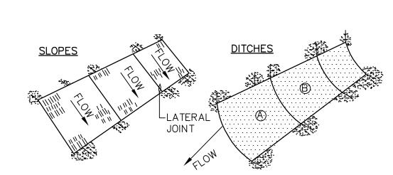
1. BURY THE TOP END OF THE MESH MATERIAL IN A 6" TRENCH AND BACKFILL AND TAMP TRENCHING SECURE END WITH STAPLES AT 6" SPACING, 4" DOWN FROM EXPOSED END.
