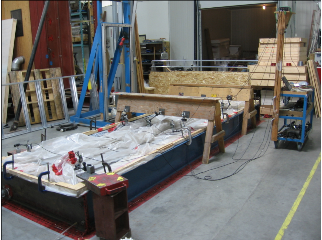
Photo 1. Transverse Load Test Set-up
