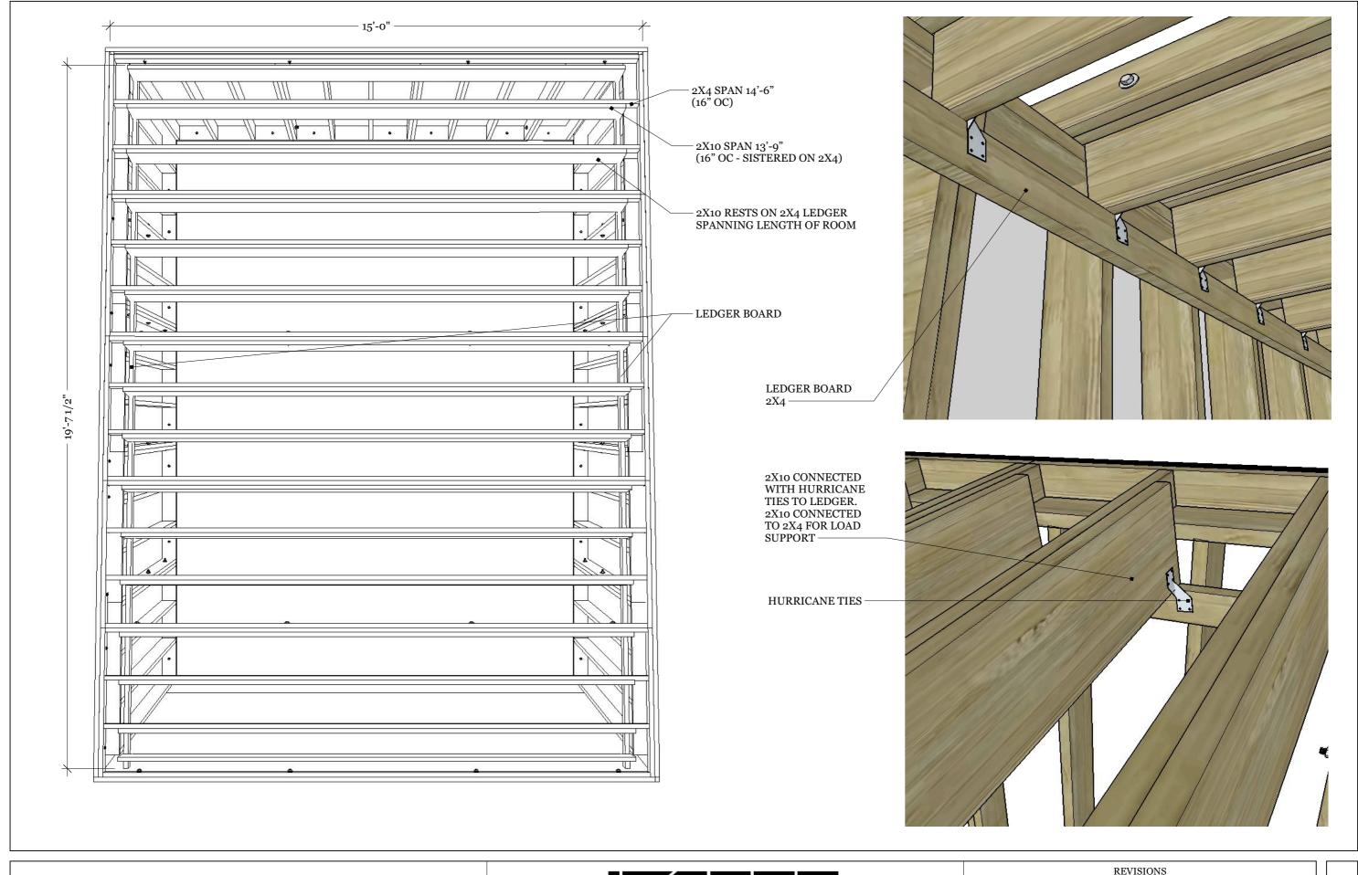
ICE RESURFACER STRUCTURE FRAMING / ROOF
