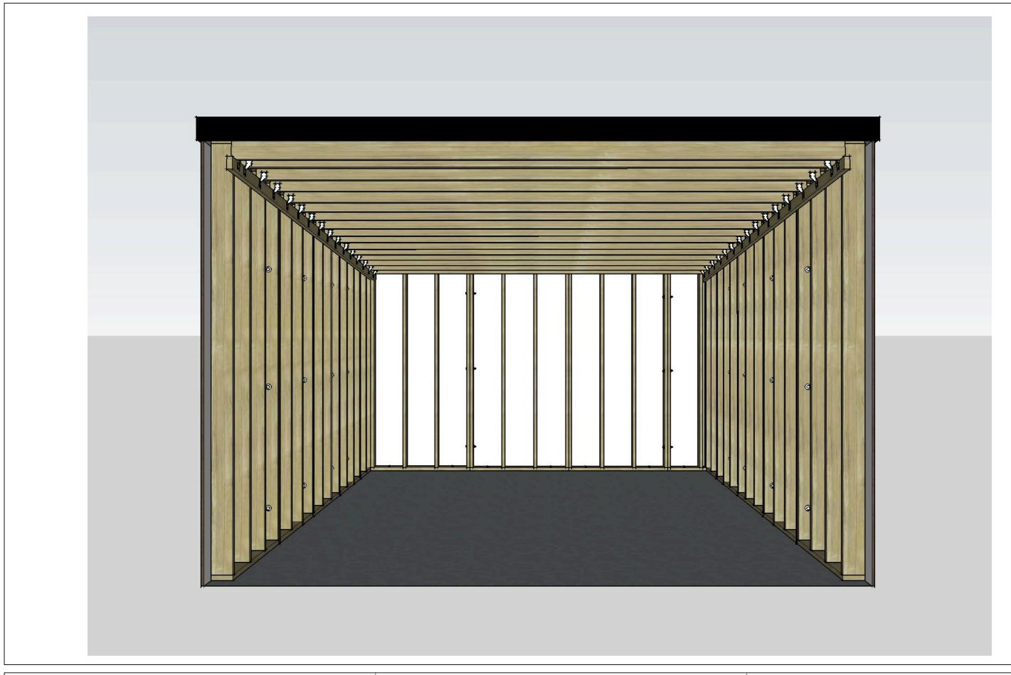
ICE RESURFACER STRUCTURE FRAMING / ROOF
