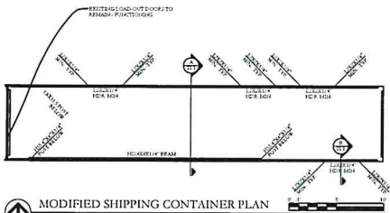
MODIFIED SHIPPING CONTAINER PLAN NOTES: 1. SHIPPING CONTAINERS ARE TO BE STRUCTURALLY SOUND WITHOUT MAJOR DENTS OR SUBSTANTIAL RUST TO FRAMES OR STRUCTURAL METAL MEMBERS. SCALE 1/4"=1'-0"
