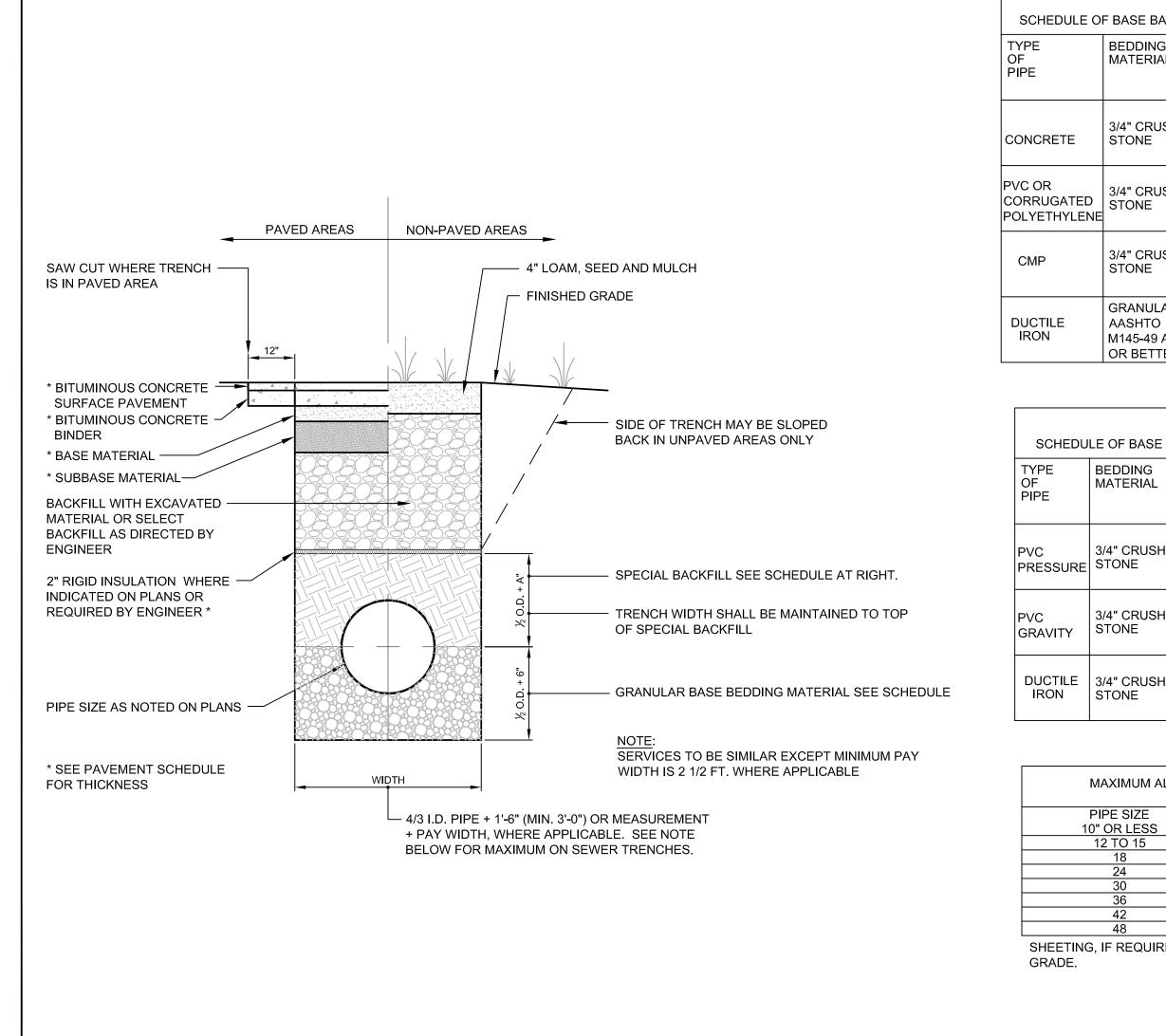
TYPICAL SEWER, WATER MAIN, AND STORM DRAIN TRENCH SECTION
