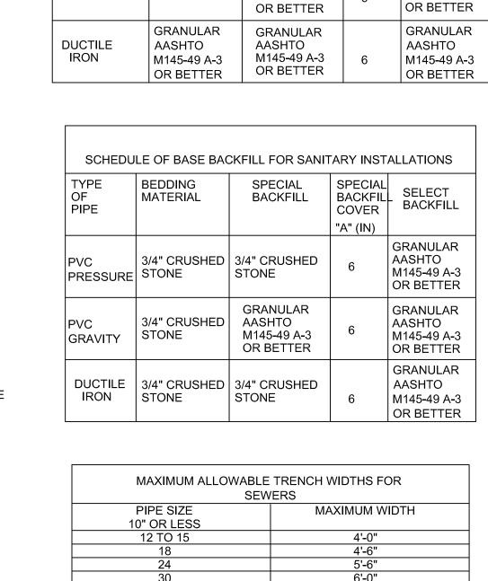
SCHEDULE OF BASE BACKFILL FOR NON-SANITARY INSTALLATIONS
