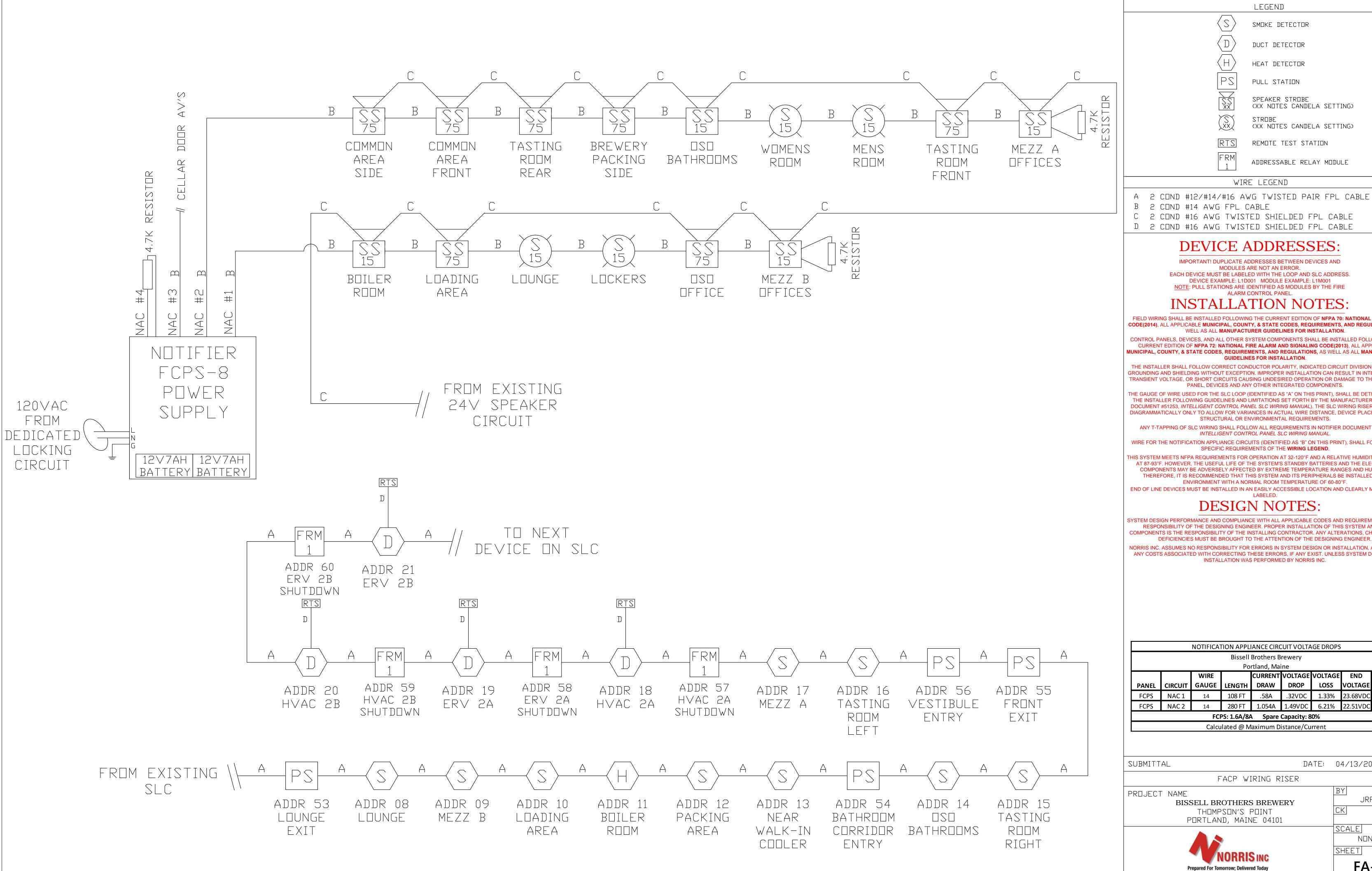
SMOKE DETECTOR DUCT DETECTOR HEAT DETECTOR PULL STATION SPEAKER STROBE (XX NOTES CANDELA SETTING) STROBE (XX NOTES CANDELA SETTING) REMOTE TEST STATION ADDRESSABLE RELAY MODULE WIRE LEGEND
