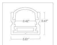
IQA-VEGA - Profile Aluminum Extrusions Max Length: 98.25 in Dimension: .61 in x .47 in Material: Anodized Aluminum Cover Options: Frosted (FL) including frosted end caps Beam: 15-20, 50, 60, 80, 90 Fits: IP20, IP54, IP67 Screws for Clips: 0.70" in length
