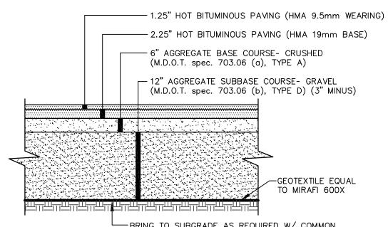
BRING TO SUBGRADE AS REQUIRED W/ COMMON BORROW COMPACTED TO 90% OF MAXIMUM DENSITY I. COMPACT GRAVEL SUBBASE, BASE COURSE TO 95% OF MAXIMUM DENSITY USING HEAVY ROLLER COMPACTION.
