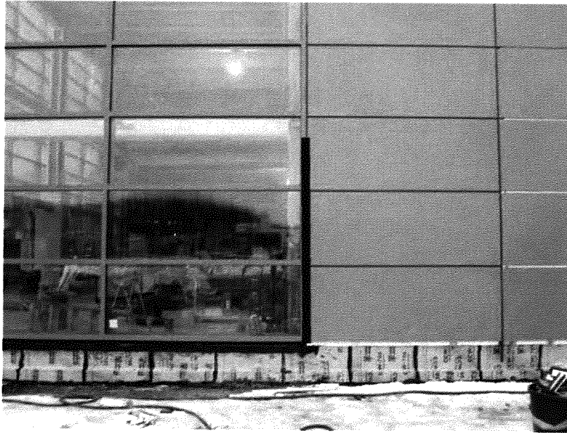
Photo No. 3 Test Specimen #2 Exterior View of Specimen with Test Area Highlighted
