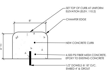
DETAIL B1 - NEW CONCRETE CURB - ALTERNATE "A'
