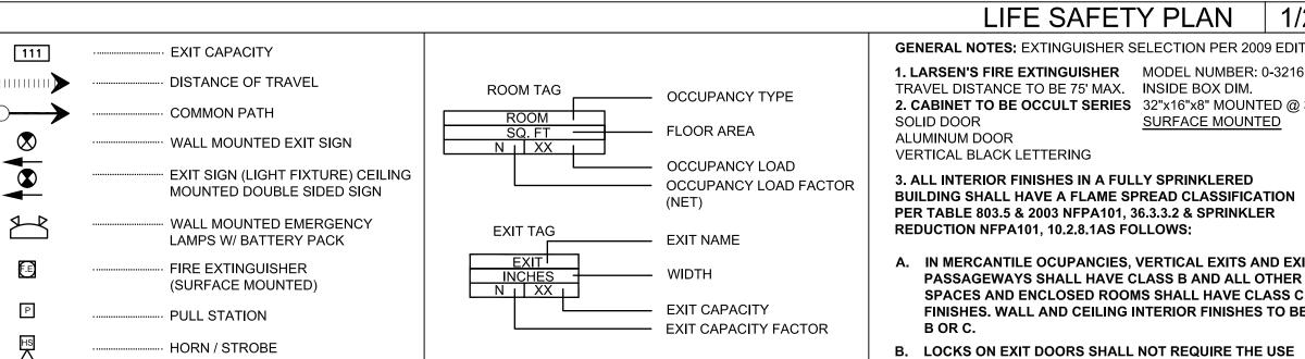
LIFE SAFETY PLAN 1/2" = 1'-0" **GENERAL NOTES:** EXTINGUISHER SELECTION PER 2009 EDITION NFPA 10 **1. LARSEN'S FIRE EXTINGUISHER** MODEL NUMBER: 0-3216 TRAVEL DISTANCE TO BE 75' MAX. INSIDE BOX DIM. 2. CABINET TO BE OCCULT SERIES 32"x16"x8" MOUNTED @ 30"A.F.F
