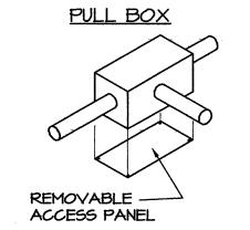
\* WHEN A JUNCTION OR MULTIPLE CHANGES IN DIRECTION ARE REQUIRED INSTALL A PULL BOX. PULL BOXES ARE TO BE INSTALLED WITH ACCESS PANEL ON THE UNDERSIDE OF THE BOX AS ILLUSTRATED.
