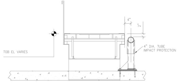
**A** DETAIL SECTION - IMPACT PROTECTION AT FLAT PLATE DEVICE
