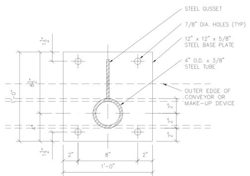
**2** DETAIL SECTION - IMPACT PROTECTION BASE PLATE AND POST
