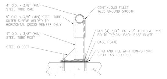
**3** DETAIL SECTION - IMPACT PROTECTION FLOOR LEVEL
