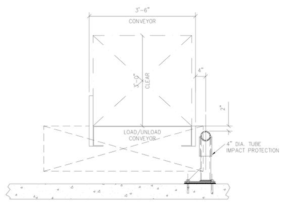
**B** DETAIL SECTION - IMPACT PROTECTION AT LOAD-UNLOAD CONVEYORS
