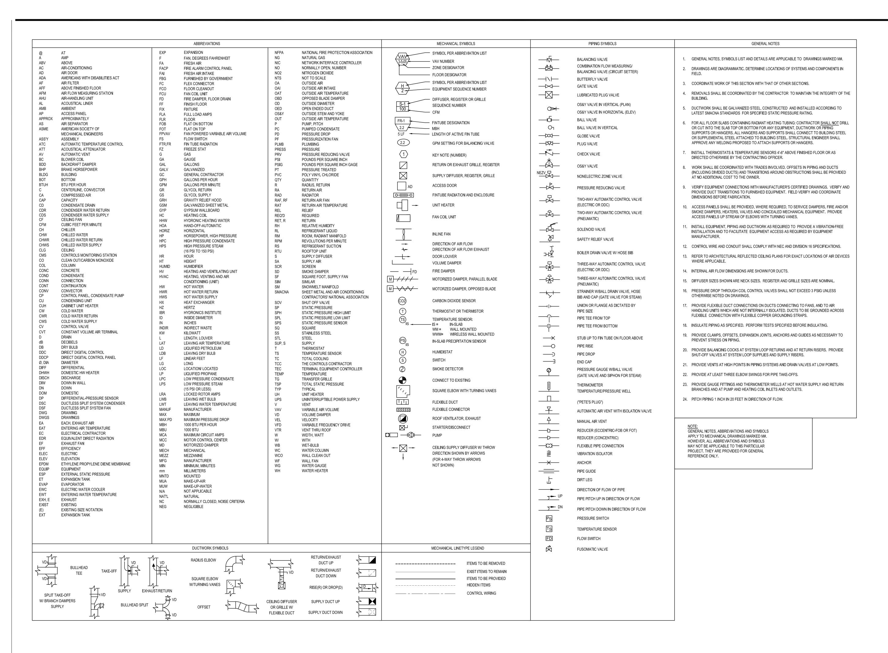
CONTROL LEGEND ANALOG INPUT **ANALOG OUTPUT** DIGITAL INPUT DIGITAL OUTPUT ACTUATOR TEMPERATURE SENSOR PRESSURE SENSOR RELATIVE HUMIDITY SENSOR AIRFLOW MONITORING STATION SMOKE DETECTOR VARIABLE SPEED DRIVE STARTER/CONTACTOR CONTROL DAMPER CONTROL VALVE - TWO WAY CONTROL VALVE - THREE WAY CIRCULATING PUMP RELATIVE HUMIDITY SENSOR
