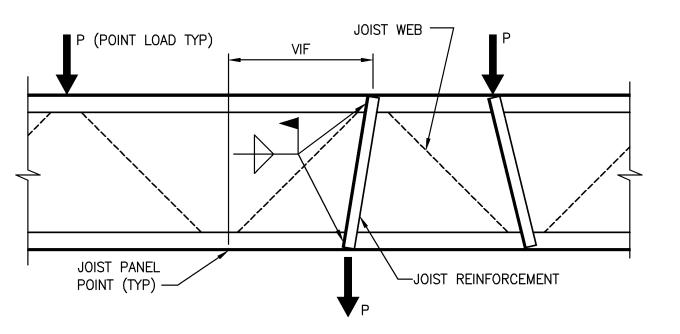
NOTE: ALL POINT LOADS ON JOISTS SHALL BE AT PANEL POINTS, OR JOISTS SHALL HAVE WEB REINF AS SHOWN FOR POINT LOADS BETWEEN PANEL POINTS
