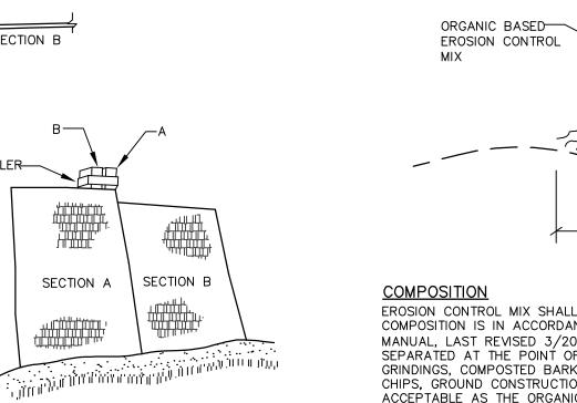
**INSTALLATION:** 1. EXCAVATE A 6"x 6" TRENCH ALONG THE LINE OF PLACEMENT FOR THE FILTER BARRIER.
