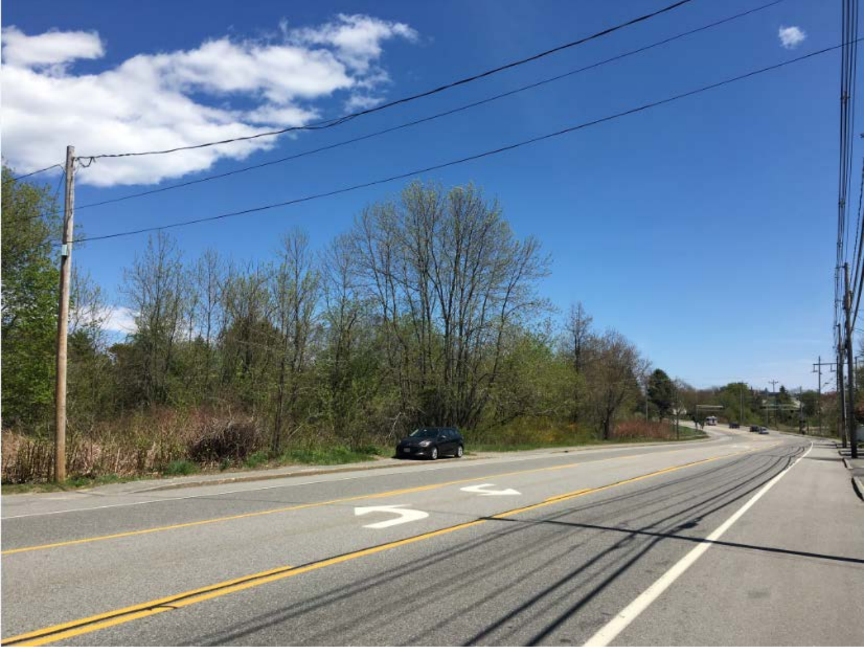
Looking east down Congress. Note pole line on opposite side but room to place second pole on eastern edge for dual telco paths.
