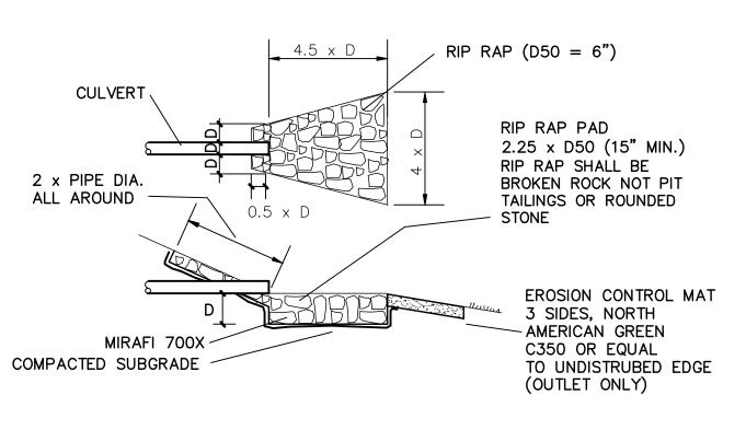
PIPE INLET/OUTLET PROTECTION
