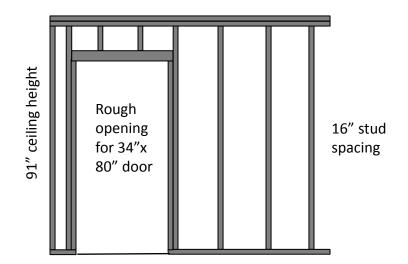
Rear wall with rough opening for 34"x80" steel insulated prehung exterior door
