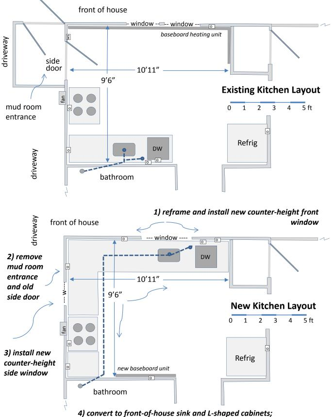
reconfigure plumbing, reposition heating unit and modify existing 14/3 grounded wiring and GFI outlets
