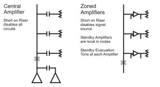
Because all EST3 zoned amplifiers have an integrated backup 1000 Hz temporal tone generator, the locally-generated alarm tones notify occupants of a hazard – even with the primary riser out of commission. The backup tone also operates if the ASU or the audio distribution system fails. To further enhance system survivability, a single standby amplifier can backup any zoned amplifier in the same cabinet.
