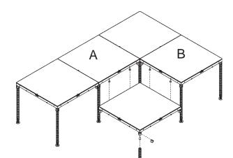
A. Insert one leg in corner socket as shown and set stage section down over connecting pins.
