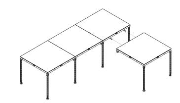
The first stage section in additional rows is attached in the same manner as the stage sections in the first row, using two legs in the sockets as shown. Each additional stage section must be pinned through the sockets to the adjoining stage sections.
