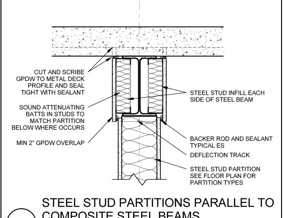
COMPOSITE STEEL BEAMS SCALE: 1 1/2" = 1'-0"
