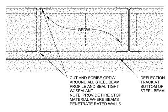
**ELEVATION - PARTITION** PERPENDICULAR TO STEEL BEAMS SCALE: 1 1/2" = 1'-0"
