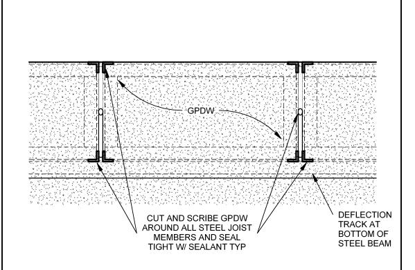
**ELEVATION - PARTITION** PERPENDICULAR TO STELE JOIST SCALE: 1 1/2" = 1'-0"
