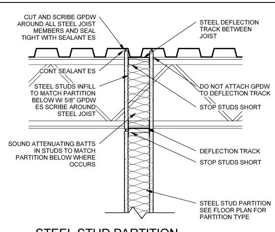
STEEL STUD PARTITION \ PERPENDICULAR TO STEEL JOISTS SCALE: 1 1/2" = 1'-0"
