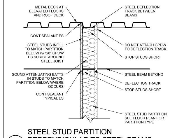
B5 PERPENDICULAR TO STEEL BEAMS
