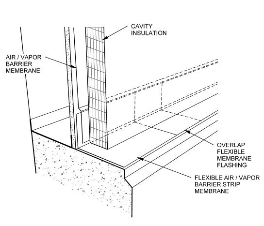
BASE OF WALL FLASHING DETAIL
