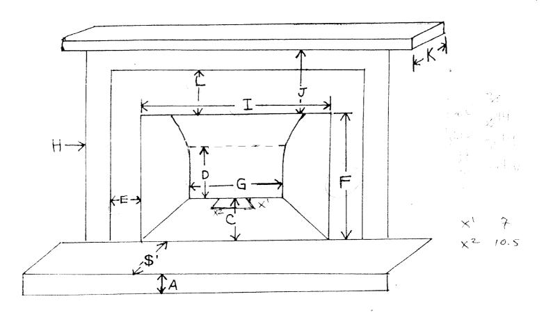
A HEIGHT OF HEARTH min 16 B DEPTH OF HEARTH DEPTH OF FIREPLACE HEIGHT OF FIREPLACE IN BACK DISTANCE OF WOOD TRIM FROM EDGE OF FP HEIGHT OF FP OPENING 31.45 (5)= WIDTH OF FP IN BACK 20.256 HOW MUCH POES THE TRIM STICK OUT H WIDTH OF FP OPENING 30 HEIGHT OF FP OPENING TO MANTEL 24.500 MEASURE THE DEPTH OF MANTEL ON UNDER SIDE MEASURE FROM TOP OF FP TO NEAREST 9.45 JEST
