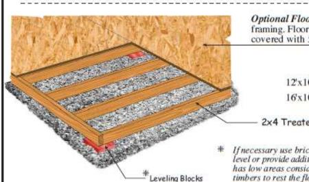
Optional Floor: is constructed with treated 2x4 framing. Floor joists are spaced 16" on center and covered with 5/8" OSB (oriented strand board).
