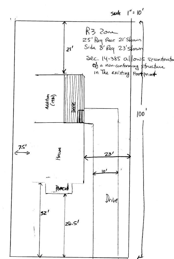
38 Hastings Street 20'x 8' decke re-build existing Framing Ledgen: 2x8 attached w/lag screws to sill DOOR Joists 2x8x8 = joist each end 4x4posts on concrete foothors (6" diameter) 46" 4160 2 steps: re Railing 30 " high 2-248 Roon height = ono more Than Blutand Max dist bet posts 8' joist / 4x8 beam: 9' Troad Depta: at least 100 (using decking x2) If combo 736" Total Ase = 22" O"tread Guardrails to the main as Existing- no damage w bracket or 36" combo
