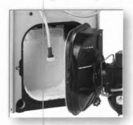
The full swing-away burner door provides easy access to the entire combustion area to simplify inspection, cleaning and burner servicing. If desired, the door can be easily removed from the hinges. A quick-disconnect plug breaks power to burner when door is open.
