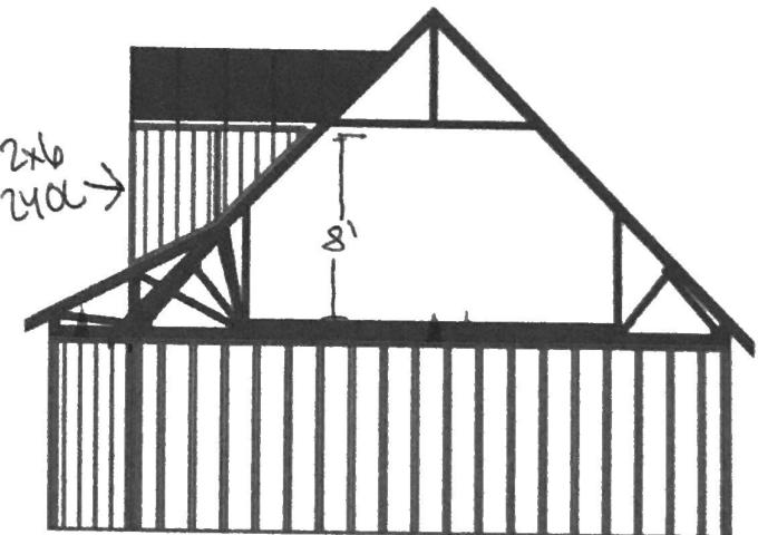
The main trusses have been installed. Due to a stairwell we had to double up trusses on either side creating a gap in the trusses. Mainly trusses have designed this dog house dormer for us. The walls are 2x6 24OC per their specifications. The trusses will sit on a double 2x6 top plate 24OC. I have provided the nailing plan for existing trusses to meet their specs. Dormer matches 12 pitch of rest of roof and so does overhangs.
