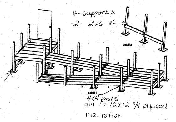
Note: The same options for transition to the ground are used for this design. Guardrail/handrail options are also the same except the inside guardrail on the lower portion of the ramp will be attached to the center 4x4's. Between modules 3 & 4 some 2x2x30 spindles will need to be screwed in place from inside the ramp.
