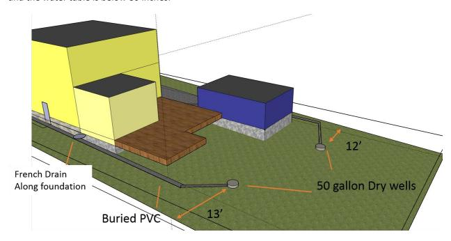
On the East side of the house is the gravel driveway and garage. Along with the French drain I will install a drain grate perpendicular to the drive, just above the garage. This will lead into a French drain that follows along the garage foundation. Buried PVC pipes will lead the water into the dry well in the backyard.
