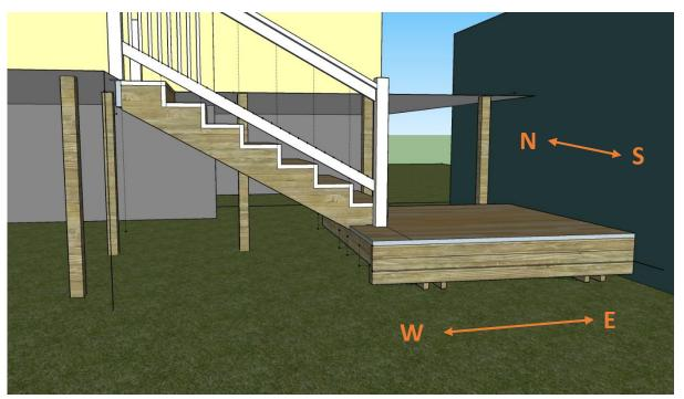
Area under new deck will be back filled to level, then it will slope to back yard South
