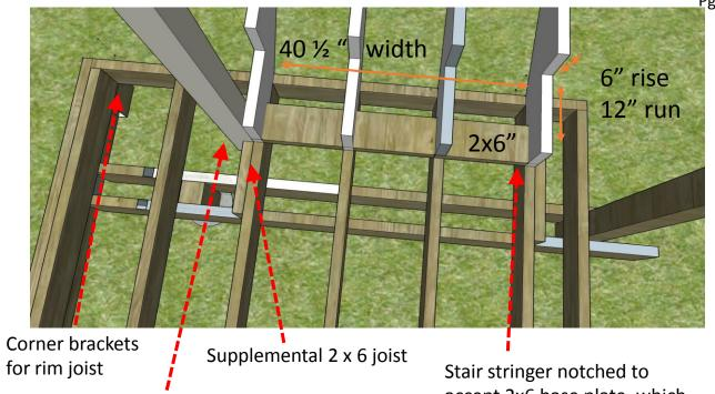
Post for handrail/guardrail notched for supplemental joist with carriage bolt through both joists and post. Additional carriage bolt through post and stair stringer Stair stringer notched to accept 2x6 base plate, which is anchored to joists
