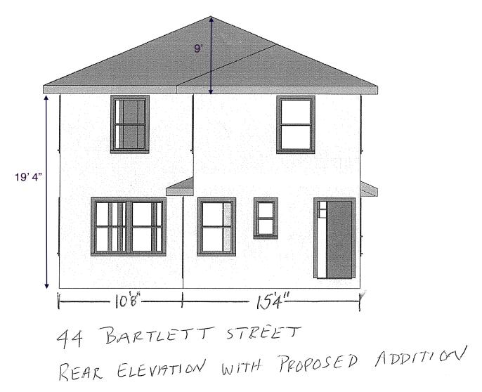
Elevation dimensions include 2'4" foundation height. Drafting software does not draw foundations.
