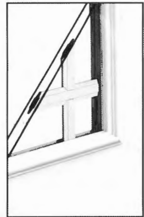
Grilles Between the Glass (GBG)
