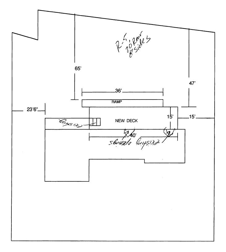
FRAMING; 2X8 PT, 16" ON CENTER - 7/2' Spon OK DECKING; 5/4 PT RAILINGS; 42" HIGH, SPINDLES 4" ON CENTER RAMP; APPROXIMATELY A 36" DROP. 1.5" ROUND HAND RAIL
