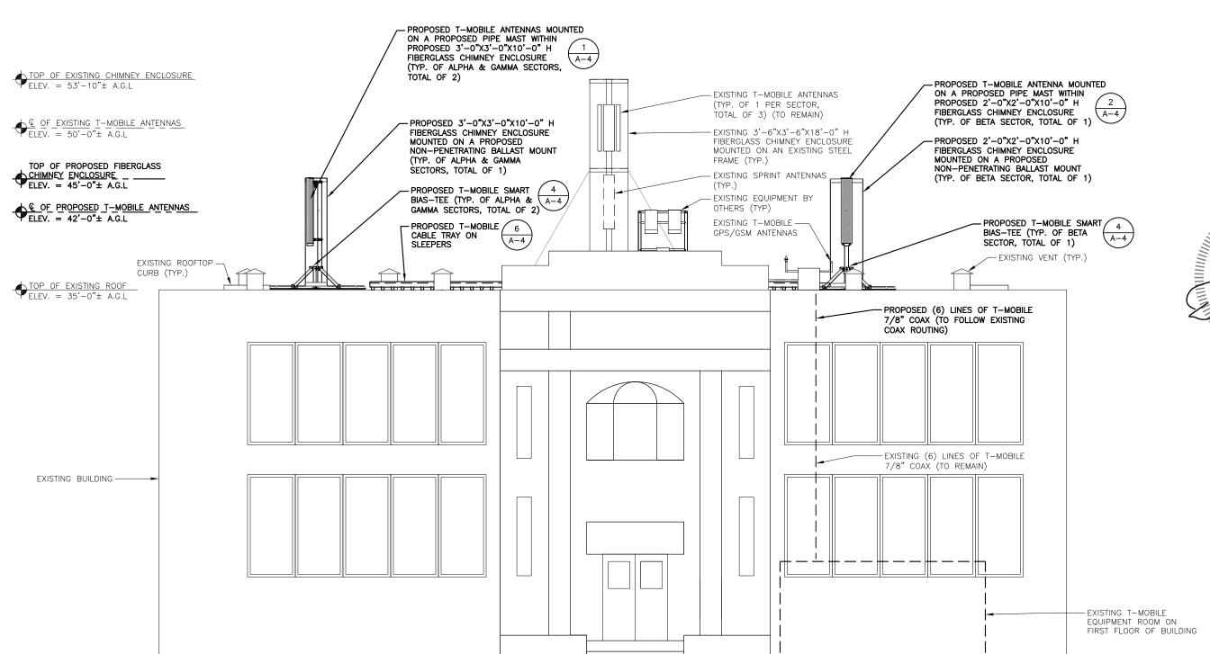
**EAST ELEVATION** 22x34 SCALE: 1/4"=1'-0"
