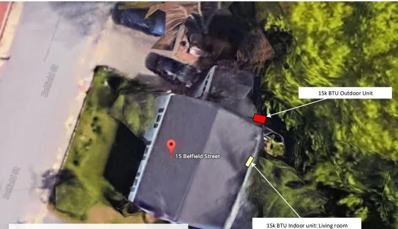
Outdoor Unit (1) Mitsubishi MUZ-FH15 - 124 lbs Installation: Exterior wall bracket Location: Surface mount
