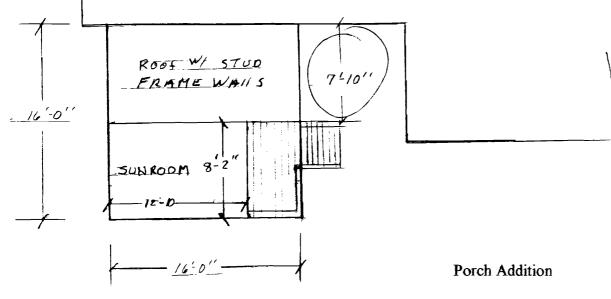
Floor System: To be constructed of 2x10 wood joists
